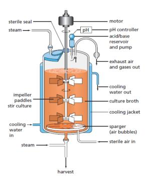
An industrial fermenter can be used to culture micro-organisms on a large scale. Sensors are used to monitor temperature, pH and oxygen levels.
